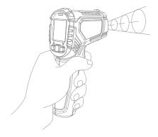
Non-contact temperature measurement includes two measurement modes, normal measurement and maximum measurement,
